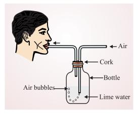
Fig. 15.1 : Testing presence of CO<sub>2</sub> in air
