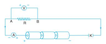
Fig. 8.2 (c) Circuit Diagram with three cells
