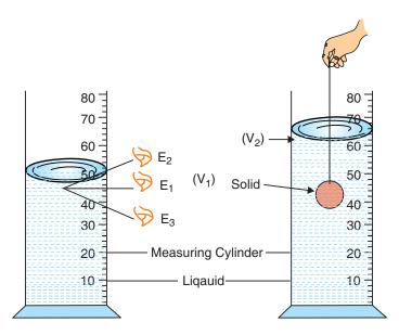
Fig. 1.2: Reading level of liquid in *a measuring cylinder*
