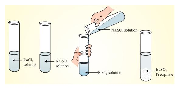
Fig. 20.4 Double displacement reaction between BaCl<sub>2</sub> and Na<sub>2</sub>SO<sub>4</sub>
