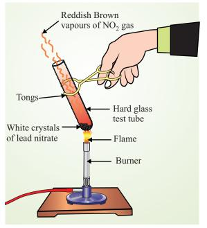
Fig. 20.2 Heating of lead nitrate
