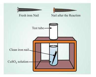
Fig. 20.3 Displacement reaction between iron and CuSO4 Solution
