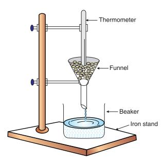
Fig. 5.1: Experimental set up for finding melting point of ice
