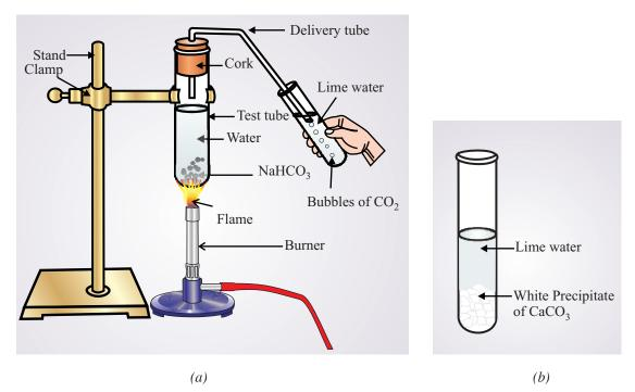
**Fig. 19.1:** (a) Heating of baking soda and passing the  $CO_2$  produced through lime water (b) Formation of white ppt. of  $CaCO_3$
