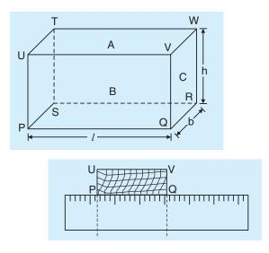
Fig. 3.3: Positioning the cuboid along the scale
