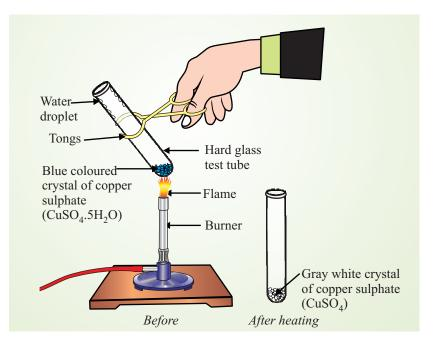
Fig. 14.2 Heating of CuSO<sub>4</sub>.5H<sub>2</sub>O
